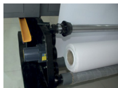
Deposited mode by holding media with 2 rollers
